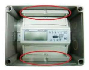
2. Pull the locking pins away from the energy meter.
