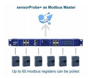
In Master mode, you can poll Slave devices via Modbus device IDs over Modbus RTU or TCP/IP.
