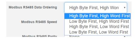
Additionally you have the option to define the data ordering from the drop-down list. **Important:** Please note the warning messages when enabling RS485 support:
