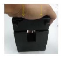
3. To reassemble the transformer, also remember to depress it firmly once again before reinserting the 2 bolts back in place. See image below.
