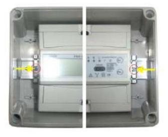
Slide out the top and bottom wiring shield using both hands.
